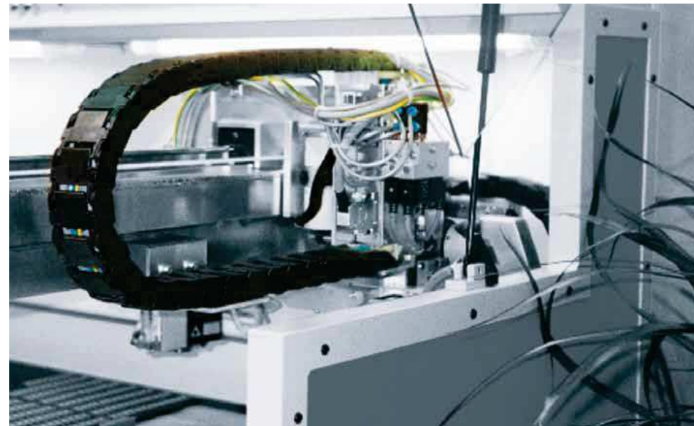
igus® zipper e-chain® series 15 in a special purpose machine for quick cable installation
