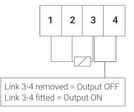
Terminals 1 to 3 allow for the connection of a three wire PT100 sensor. Terminals 3 to 4 allow the user to select the default heating status on sensor error. Without a link fitted the heating will turn OFF if a sensor error is detected (default). With a link fitted the heating will turn ON if a sensor error is detected
