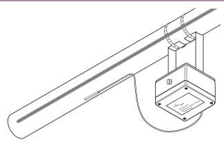
nVent RAYCHEM ETS-05 electronic surface and ambient sensing thermostat provides accurate temperature control for heating cables.
