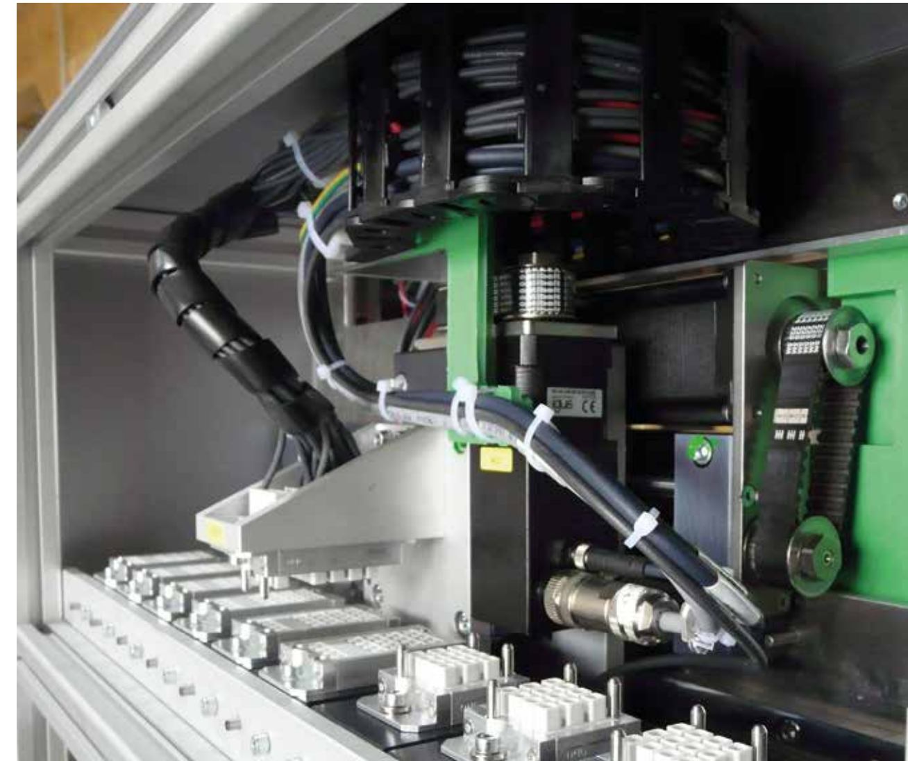
chainflex® CF31 motor cable in a fast pick-and-place machine
